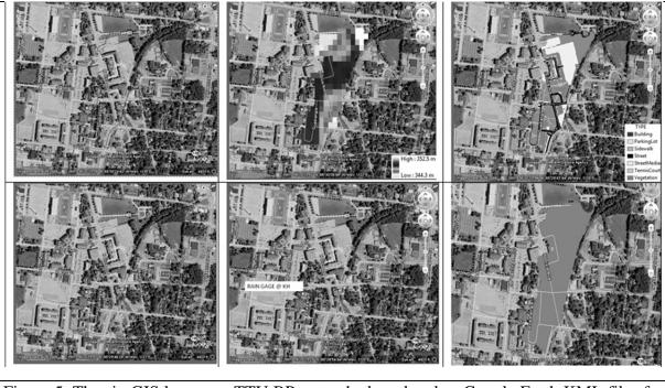
Figure 5. The six GIS layers on TTU BP watershed rendered as Google Earth KML files for display in HydroViz-TTU adaptation. Each layer in a panel represents a hydrology topic. From upper left (clockwise): General watershed boundary, elevation/terrain, land use/land cover; watershed outlet, instrumentation and soil coverage.
