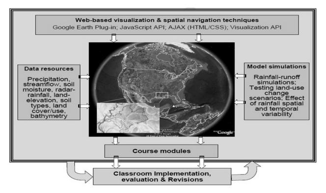
Figure 2. Overall architecture of HydroViz developed by Habib et al.[5] depicting the various inputs and modules. (*figure reprinted with kind permission from Habib et al.* (2011))
