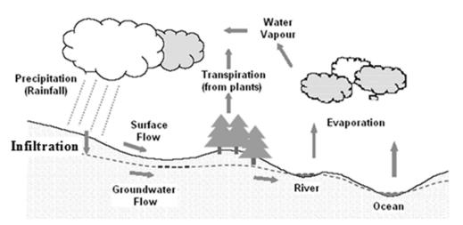
Figure 1. Overview of the major processes of the water cycle that are important to the engineer for design and operations of water resources systems.
