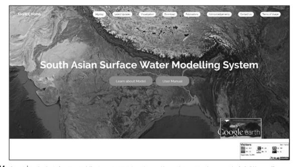
Q14 Figure 3 | South Asian Surface Water Modelling System (SASWMS; http://depts.washington.edu/saswe) Portal as an example of a 'build-it-yourself' open source web interface connecting a complex back-end model (VIC model in this case) for enabling water management decisions.
