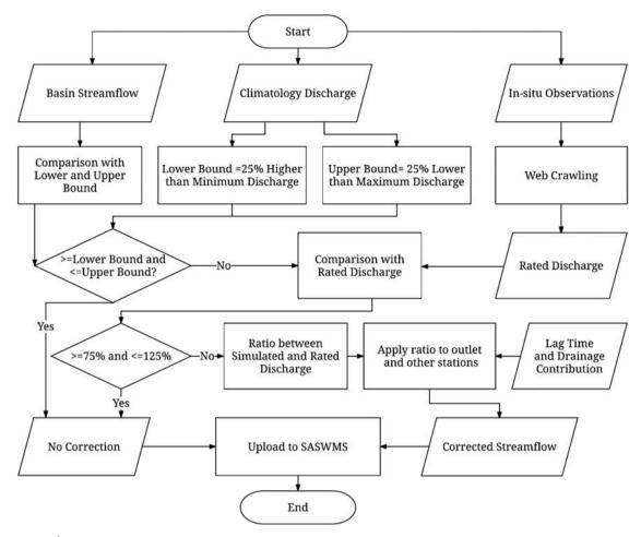
Figure 7 | Flow chart of streamflow correction system.
