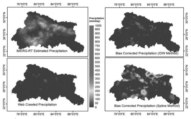
Figure 12 | Example of correction of IMERG-RT precipitation of 1st July 2016 of Ganges Basin, upper left: IMERG-RT precipitation, upper right: corrected precipitation by IDW method of bias interpolation, lower left: web crawled precipitation and lower right: corrected precipitation by spline method of bias interpolation.
