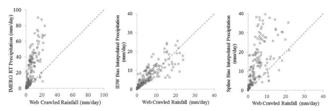
Q17 Figure 10 | Scatter plot of daily cell average precipitation of Brahmaputra Basin between interpolated web crawled rainfall and left: IMERG-RT precipitation, middle: Bias corrected precipitation by using IDW method of interpolation and right: Bias corrected precipitation by using spline method of interpolation.
