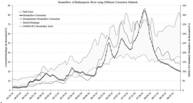
Q21 Figure 16 | Comparison of dynamic correction procedures for the Brahmaputra Basin with uncorrected precipitation. Rated discharge is the discharge derived from observed water levels.
