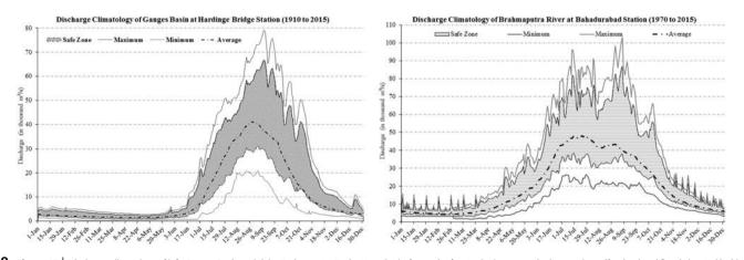
Q20 Figure 15 | Discharge climatology of left: Ganges Basin and right: Brahmaputra Basin. Here the 'safe zone' refers to the 'no-correction' zone where, if a simulated flow is located inside, no automatic checks will be triggered.
