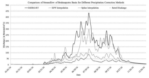
**Q18** Figure 11 | Comparison of simulated streamflow of Brahmaputra Basin from different types of precipitation.
