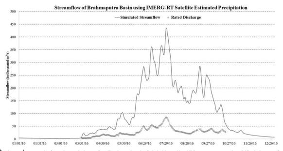
Q12 Figure 1 | An example of poor data quality issues of satellite observations that limit decision making skill for water managers. The solid line is the streamflow simulation derived from a hydrologic model forced with GPM's IMERG satellite precipitation data. The dotted red line is the observed discharge rated from water levels. (source: http://depts.washington.edu/saswe).
