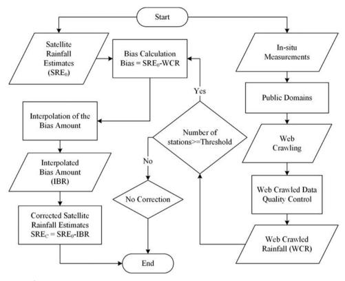
**Figure 6** Precipitation correction system flowchart.
