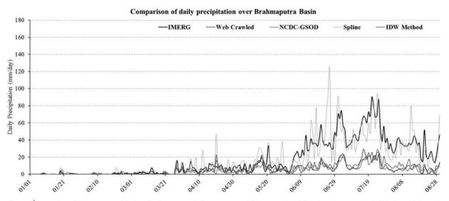
Figure 9 | Comparison of cell average precipitation of Brahmaputra Basin from IMERG-RT rainfall, corrected rainfall produced by IDW method of bias interpolation and corrected rainfall from spline method of bias interpolation.
