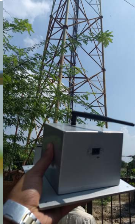
Router for LPWAN – Needs one solar panel Collects data and pushes to cloud
