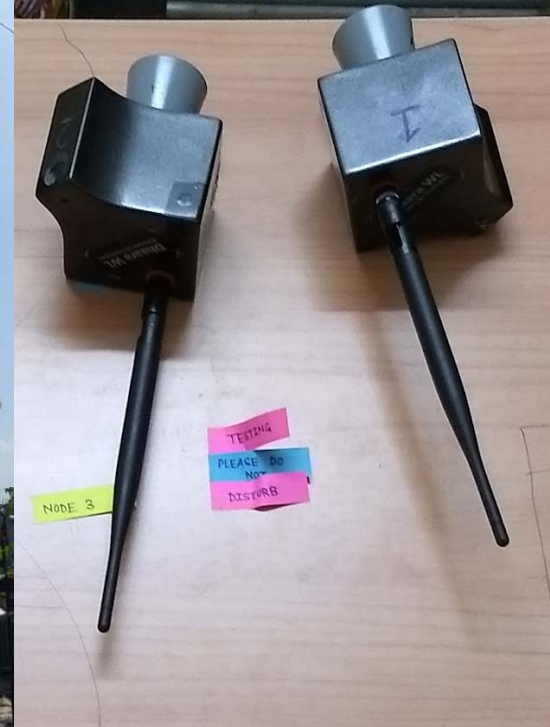
IoT sensors- Runs on 2 AA batteries- for 2 years
