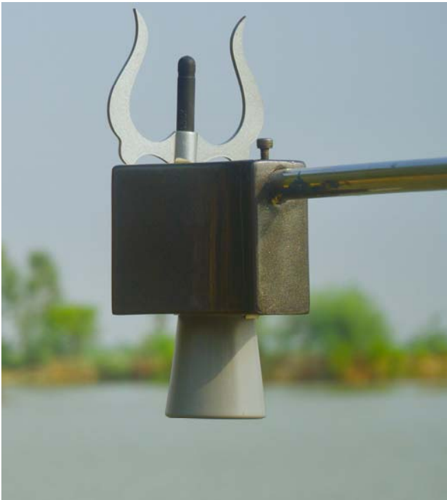
IoT compatible water level sensor – Runs on 2 AA batteries for 2 years
